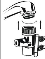
3. Screw the diverter valve onto the faucet, turning swivel collar to tighten (Fig. 3).
