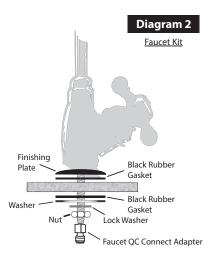
It may be necessary to drill a hole 7/16" in diameter through the sink or countertop
