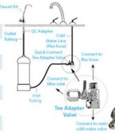
Installation kit includes 6 feet of tubing (1/4" outside diameter, longreach faucet, fittings and adapters 17.25" (43.82 cm) including fitting
